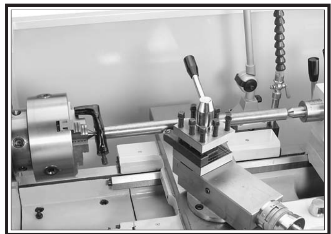
Figure 53. Example photo of a workpiece mounted between the centers.
